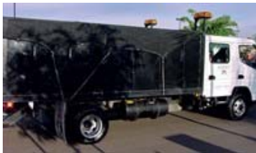
Large capacity trucks, such as this Mitsubishi Fuso, can transport and haul large volumes of debris, and overhead warning lights help keep other drivers and the crew safer.
