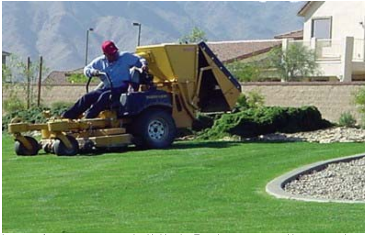
Large turf areas are managed with Hustler Z series mowers and large capacity catchers for winter ryegrass that is traditionally too wet to mulch.
